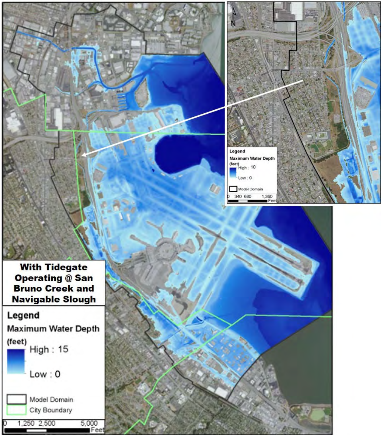
Figure 4-4: Flood Extents with Operational Tidegate at San Bruno Creek and Navigable Slough
