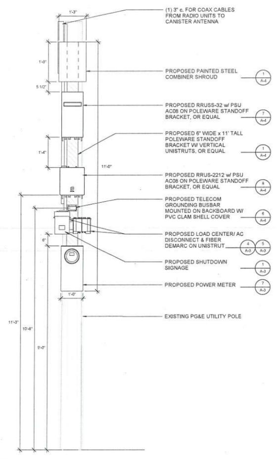
1 ENLARGED EQUIPMENT ELEVATION
