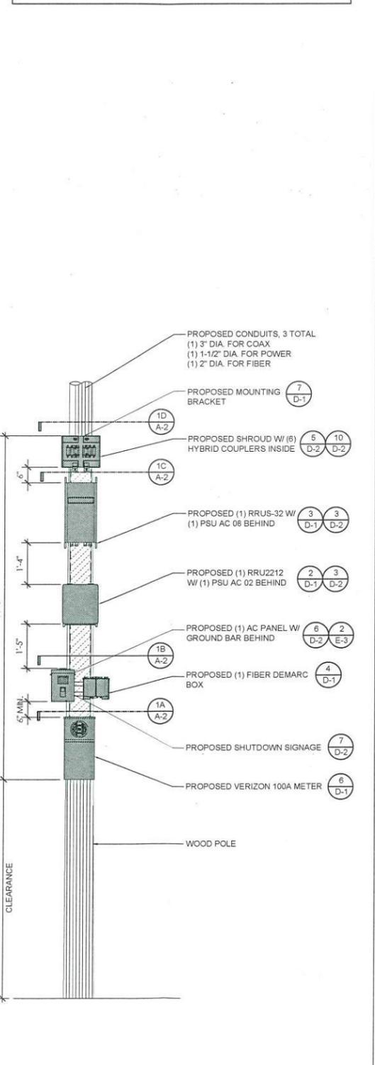
PROPOSED ELEVATION 24"x36" SCALE: NTS 11"x17" SCALE: NTS 2
