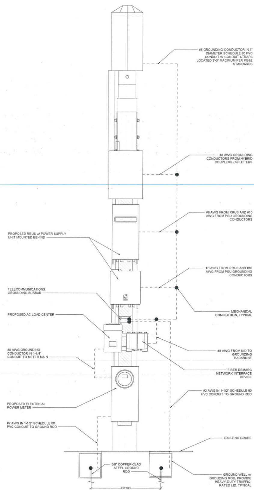
NOTE: REFER TO ELEVATIONS FOR MOUNTING REQUIREMENTS. BOND ALL ELECTRONIC COMPONENTS TO NEW GROUNDING RING
