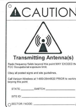
NOTE: MOUNT WARNING SIGNAGE 3'-0" BELOW PROPOSED CANISTER ANTENNA
