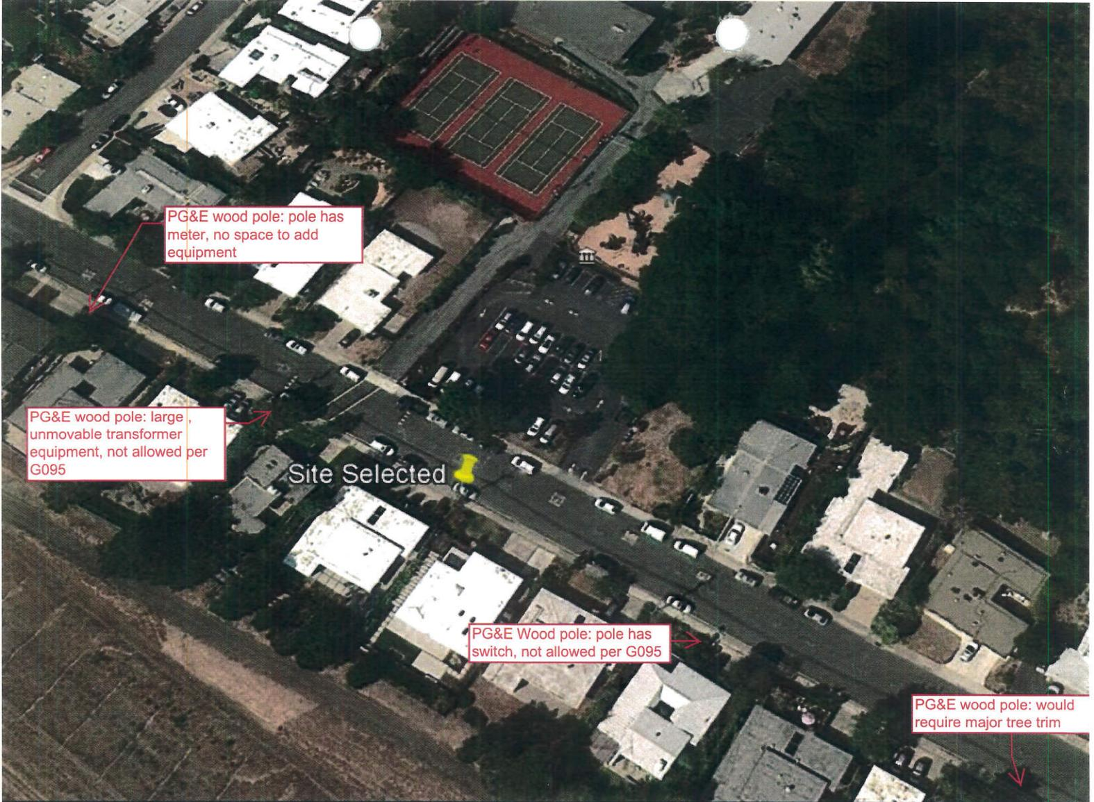
PG&E wood pole: pole has meter, no space to add equipment
