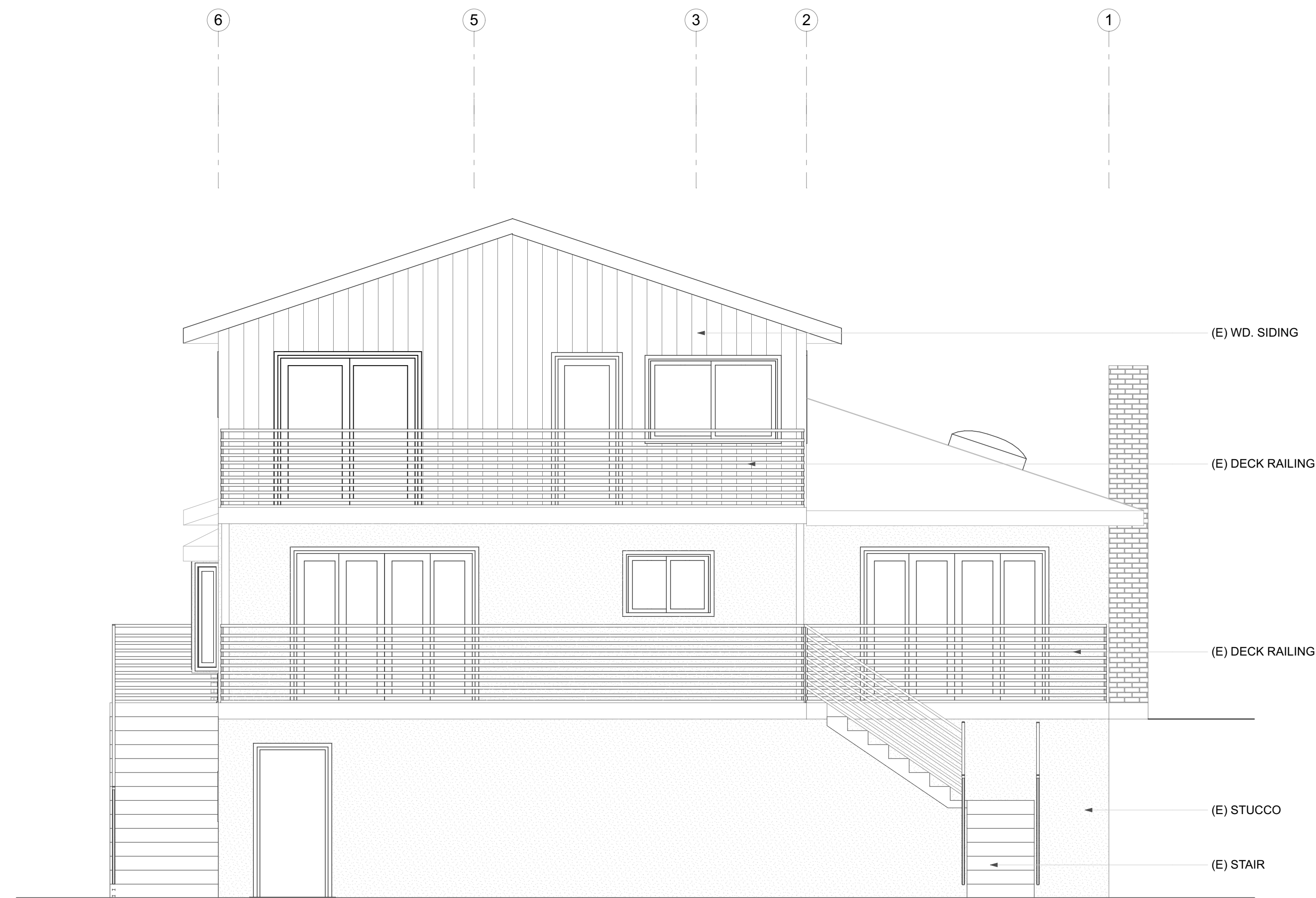
1 (E) EAST REAR ELEVATION SCALE: 1/4" = 1'-0"
